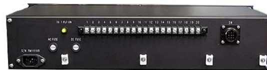
The coaxial switch plugs into the 9-pin amp connector. Transmitter and remote control connections are made to barrier strip terminals.
